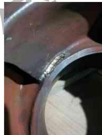
给水泵叶轮汽蚀焊补修复
